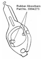
3. The release bearing guide on the front of the gearbox wears considerably, allowing the bearing to rattle on this component. To stop the fork fouling, it is necessary to remove sufficient material from the bell housing to stop the fork contacting. Whenever a clutch is replaced, inspect this area for wear. If any wear is evident, the guide must be replaced.
