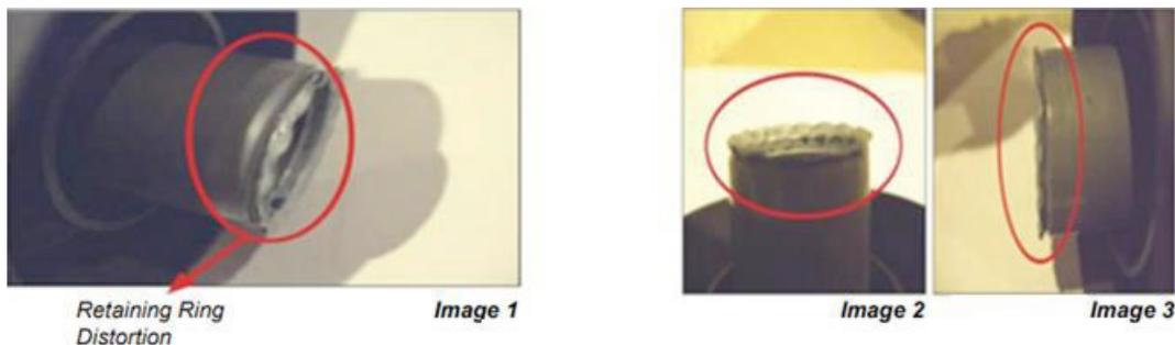
To avoid the cylinder being over-stroked, the pedal should be depressed and then released slowly to allow the cylinder to return to rest before the pedal is depressed again.
