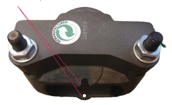
Of course old units with this kind of damage cannot be used and therefore these cannot be accepted back for credit against the surcharge
