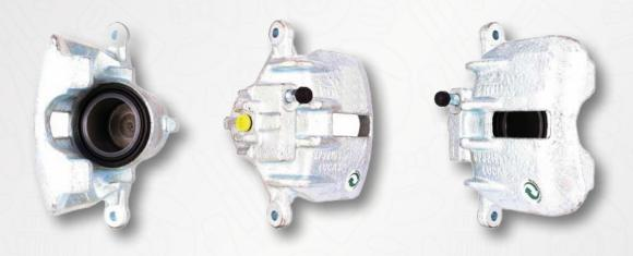
On some Honda and Rover models between 1996 and 2005, the Brake Calipers LCA150 / RCA150 can be fitted either Left hand or Right hand depending on whether the originals have been fitted as Leading (LD) or Trailing (TR) Calipers.
