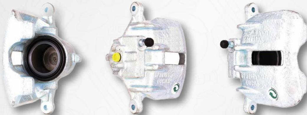
On some Honda and Rover models between 1996 and 2005, the Brake Calipers LCA150 / RCA150 can be fitted either Left hand or Right hand depending on whether the originals have been fitted as Leading (LD) or Trailing (TR) Calipers.
