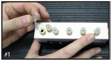
REMOVE SHIPPING PIN(S) FROM VALVE BLOCK (EXAMPLE)
