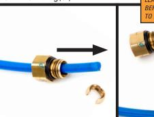
AIR LINE CAN RESULT IN POSSIBLE LEAKS. INSPECT THE AIR LINE BEFORE INSERTION. AIR LINE NEEDS TO BE REPLACED IF DAMAGED.
