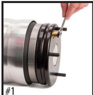
**USE A WRENCH TO LOOSEN** THREADED PLUG
