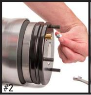
REMOVE THREADED PLUG AND DISGARD
