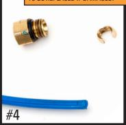
UP THE LINE AND SPREAD THE COLLET OPEN TO REMOVE
