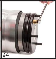
TIGHTEN FITTING TO APPROX. 2NM (18 IN-LBS/1.5 FT-LBS)
