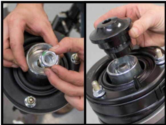
VUELVA A INSTALAR LA TUERCA Y LA COPA INFERIOR. APRIETE LA TUERCA Y VUELVA A INSTALAR LA PINZA SUPERIOR EXISTENTE.
