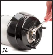
USE A WRENCH TO LOOSEN THREADED PLUG
