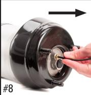
GENTLY PULL ON AIR LINE TO CONFIRM IT IS FULLY SECURED BY THE AIR LINE FITTING
