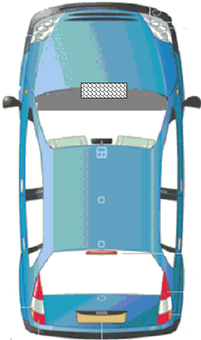
1. The Cabin Filter can be found in the engine compartment, at the base of the windscreen.
