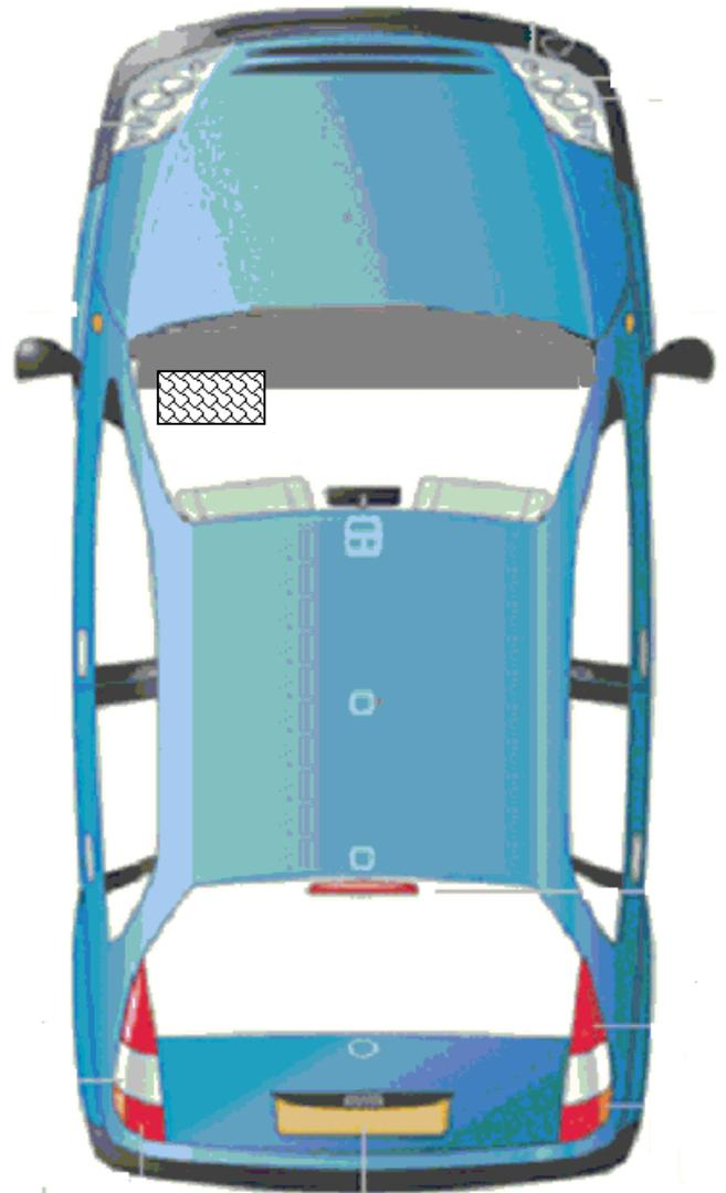
1. The Cabin Filters can be found in the ceiling of the passenger footwell.
