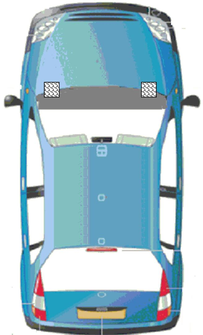
1. The Cabin Filters can be found on either side of the engine compartment near to the windscreen.
