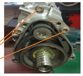
8. Screw the motor in position.
