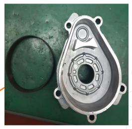
2. Carefully remove the belt from the inside of the housing, and keep safe for later use.
