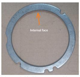
NB: when re installing the washer, ensure the grooved face is facing outwards. If fitted the wrong way around the cut outs in the washer will not line up with the black plastic bearing.
