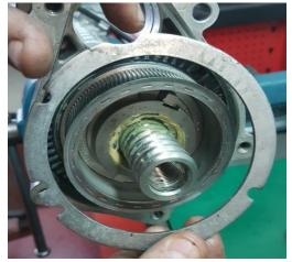
3. Carefully remove the washer, and keep safe for later use.
