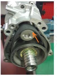
7. Hold the belt and insert the motor through the housing. Slide the belt over the teeth on the motor.
