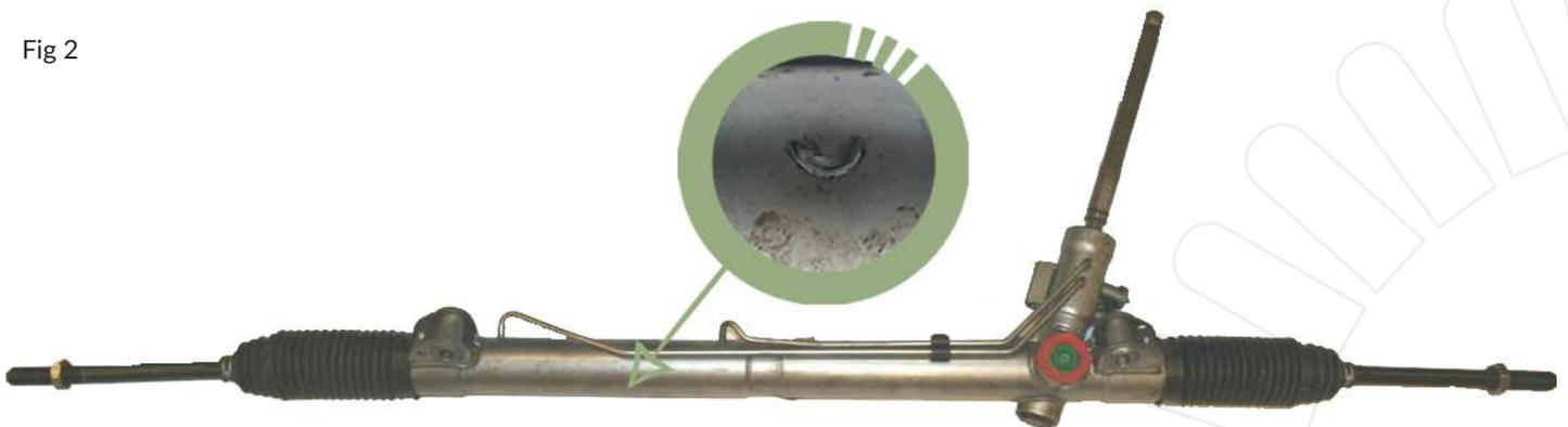
**IMPORTANT:** Please note this type of cast damage will result in a Surcharge Rejection
