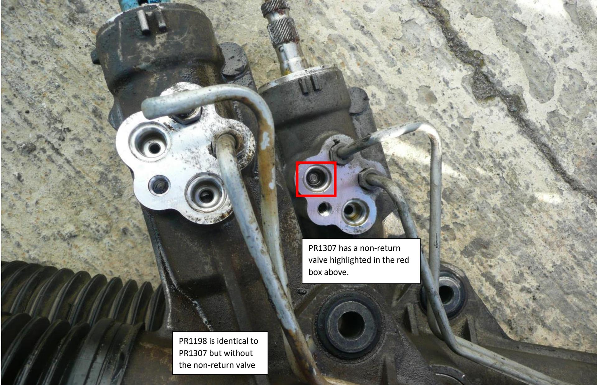
PR1307 has a non-return valve highlighted in the red box above.
