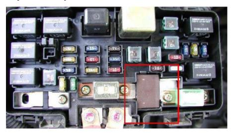
The battery sensor is built into the negative battery cable connector.
