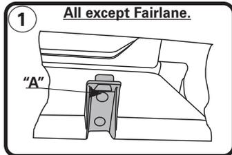
1: Place finger in channel (top centre of glove box) press down at "A", swing glove box down.
