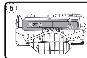
5: Install new filter cover in position, insert into the upper slot (direction A) and secure by moving the cover to the right (direction B) if fitting for first time, or use old cover. Refit all previously removed components.
