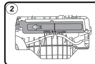
2: Slide the mesh filter or cover plate to the left to unlock.
