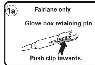
**WARNING:** Fairlane only. Retaining pin must be removed to remove glove box, depress clip as shown and remove. Failure to remove this pin will result in damage to pin.
