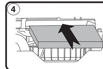
4: Slide the new filter into housing. (Position removal tab to front and on top of filter)
