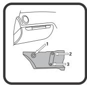
Tilter located under glovebox, remove panel by unlocking in 3 places as shown.
