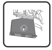
Pull dirty filter out to remove, push new Ryco filter into housing.
