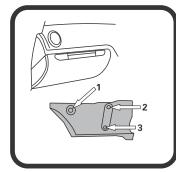
Tilter located under glovebox, remove panel by unlocking in 3 places as shown.
