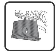
③ Pull dirty filter out to remove, push new Ryco filter into housing.
