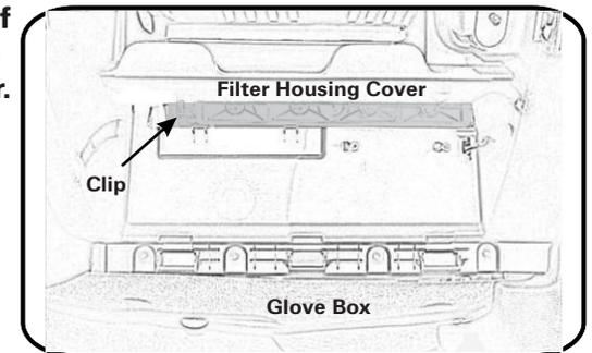
3. Replace old cabin filter with RYCO RCA242P and ensure the air flow arrow is pointing to the floor. Refit filter housing cover and glove box. Dispose of used filter correctly.
