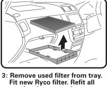
Fit new Ryco filter. Refit all previously removed components.
