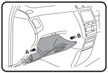
1: Push sides of glove box (A & B) to release catches, roll glove box down, unclip hinges to remove glove box.
