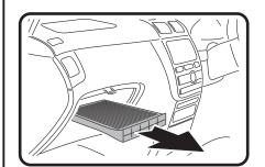
2: Slide filter tray out from glove box compartment.
