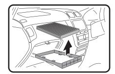
3: Remove used filter from tray. Fit new Ryco filter. Refit all previously removed components.
