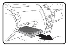
2: Slide filter tray out from glove box compartment.
