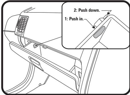
1: Open glove box and remove retaining pins on either side of glove box, then fully open glove box.
