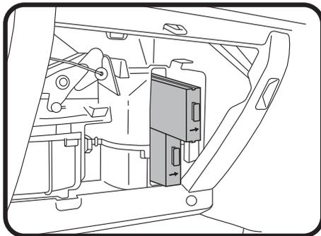
3: Remove used filters, replace with new RYCO filters (note direction of flow arrow) and reinstall all previously removed parts.
