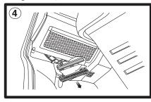
Pull filter cover down and out to remove, pull used filter out from housing.
