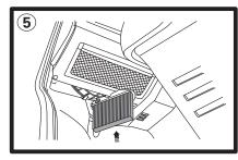
Push new Ryco RCA112P filter into housing.
