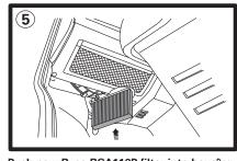
Push new Ryco RCA112P filter into housing.
