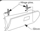
1: Open glove box, remove hinge pins by levering out as shown, remove glove box.
