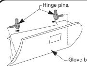
1: Open glove box, remove hinge pins by levering out as shown, remove glove box.
