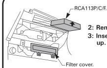
2: Remove filter cover, remove used filter.
