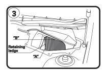
3: Ease plenum cover past bonnet, Strut, clean debris from housing. To remove mesh screen, hold at "A" with long nose pliers and move screen over retaining ledge, (Discard screen, no longer needed)
