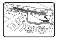
1: Starting at passenger side peel weather strip back to the end of plenum cover ("A")
