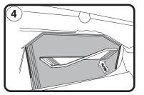
4: Clean debris from inside filter housing, Slide the new filter into housing. Filter can be twisted as shown to assist fitting to housing. Ensure filter is seated correctly behind retaining ledges.
