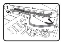
1: Starting at passenger side peel weather strip back to the end of plenum cover ("A")
