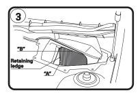
3: Ease plenum cover past bonnet, Strut, clean debris from housing. To remove mesh screen, hold at "A" with long nose pliers and move screen over retaining ledge, (Discard screen, no longer needed) To remove filter, hold pleat at "B" and pull out from top.
