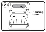
2: Remove housing cover by unclipping ends and pull out.
