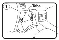
1: Partly open glove box and remove the 2 tabs, let glove box hang down out of way.
