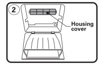
2: Remove housing cover by unclipping ends and pull out.
