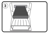
3:Remove used filter and replace with a new Ryco filter.
