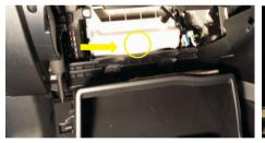
With the glove box unit out of the way the housing will be easily identifiable sitting on top of the blower fan. Remove the housing lid and pull out the dirty filter and clean area from large objects trapped in the housing.
