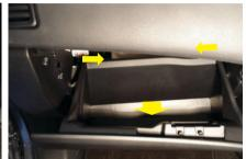
The cabin air filter housing is located behind the glovebox. To gain acces, the glovebox has to first be removed. Remove objects from compartment and unclip the strut shown in pic above.
