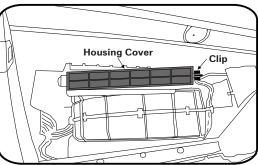
3. Remove old filter and push new filter into the housing. Refit housing cover and glove box. Dispose of used filter correctly.
