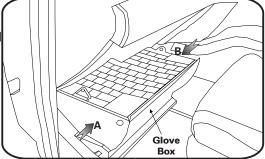
2. The cabin air filter housing is located above glove box. Remove the cover by squeezing the clip located on its right side.
