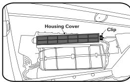
3. Remove old filter and push new filter into the housing.
