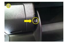
Open the glove box. With both hands positioned in both upper corners of the compartment just above the arrow on the picture, apply some force in the arrow direction to unhinge the compartment retaning lugs. Once that is done it will drop completely.
