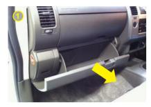
The cabin air filter is located behind the glove box on the passenger side. Please follow this instruction to replace the element.
