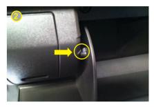
Open the glove box. With both hands positioned in both upper corners of the compartment just above the arrow on the picture, apply some force in the arrow direction to unhinge the compartment retaning lugs. Once that is done it will drop completely.
