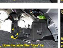
Open the cabin filter "door" by unscrewing the two philips screws
