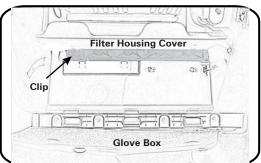
3. Replace old cabin filter with RYCO RCA242P and ensure the air flow arrow is pointing to the floor. Refit filter housing cover and glove box. Dispose of used filter correctly.
