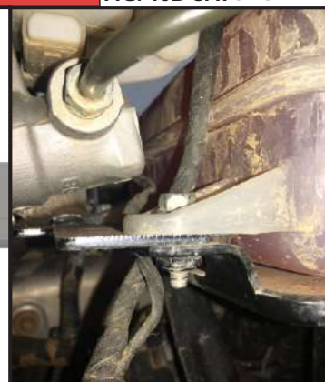
FIG. 10D CATCHCAN BRACKET INSTALLED
