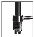
**INSTALLING THE THREADED INSERT**
