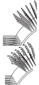
3. Mount the belts with the bent brushes in the direction of rotation.
