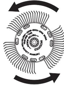
4. Assemble the two halves of the corresponding adapter through the brush belt or the eraser. Make sure that they are assembled correctly. Now place the adapter on the spindle of the sander and fix it in place with the appropriate screw. The adapter is adjusted using the inside 6-point on the spindle
