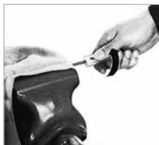
**Deburring tool can also be used with a cordless screwdriver:** Remove deburring tool cap and clamp 10 mm drive tang into the drill chuck. Proceed as described above.
