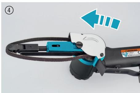
Turn cover anticlockwise to close and tighten housing screw.
