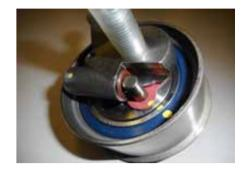
This is the correct state of the tensioner before installation. **DO NOT** install if the tensioner assembly does not resemble the image above.
