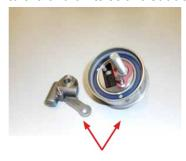
**Do not use** if hydraulic actuator has become separated from the tensioner pulley. There is an internal spring that will also need to be repositioned which can lead to premature failure if not done precisely.
