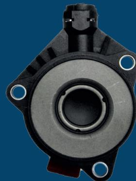
3. Once correctly fitted to the gearbox, remove the red transit clip.
