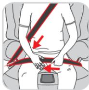
Thread the diagonal belt through the side belt guide (E) on bottom of the headrest and tighten it in the direction of the retracting mechanism. Make sure that the diagonal belt lies firmly against the child's body and is not twisted. All belts must lie tightly against the child's body without being twisted. The lap belt must lie flat over the child's thigh.
