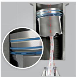
Bent connecting rods, which often occur as a result of engine damage, cause the piston to run at an angle in the cylinder. The piston rings consequently take on an elliptical form and no longer rotate in the piston. This results in uneven wear and ring flutter.
