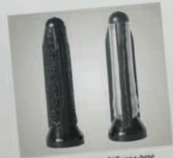
Fig. 22: Sieve filter of an E1F vane-type pump. Left: clogged - Right: new
