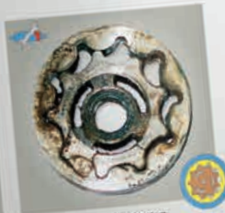
Fig. 19: A jammed pump system (trochoidal toothed ring) of an E3T toothed ring pump
