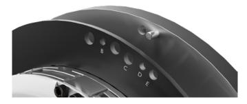
**B. Flywheel** Match holes to vehicle flywheel dowels
