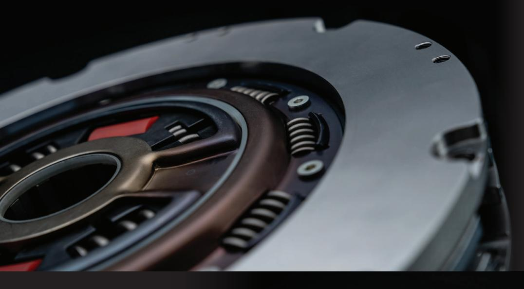
UniClutch features a patented Radial Dampening Center (RDC) which can help reduce noise and vibration in a vehicle's drivetrain by isolating the engine's rotational energy from the transmission.
