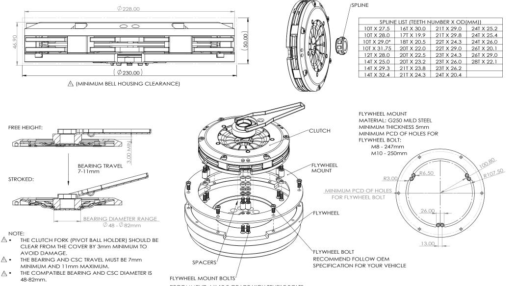
RECOMMEND 6 X 12.9 GRADE HIGH TENSILE BOLTS. IF MOUNTING TO A FLAT FLYWHEEL, USE A 60 DEGREE COUNTERSUNK BOLT WITH A CORRESPONDING COUNTERSUNK FEATURE ON THE FLYWHEEL MOUNT TO ENSURE THE BOLT HEAD IS FLUSH WITH THE UNDERSIDE OF THE FLYWHEEL MOUNT
