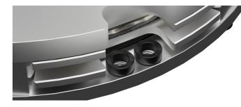
B. Add Loctite<sup>®</sup> 243<sup>™</sup> You must add Loctite<sup>®</sup> 243<sup>™</sup> to the countersunk flywheel mount bolts.
