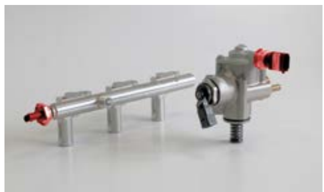
Fuel pressure sensors (highlighted) on the fuel rail and on the high-pressure pump
