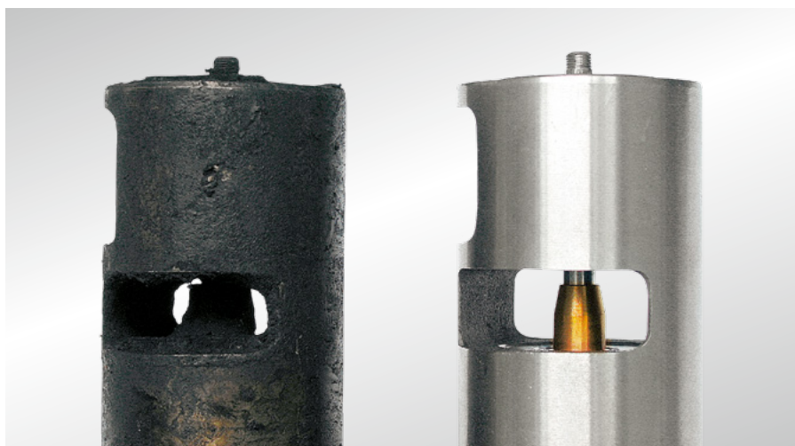
Fig. 38: EGR valve (diesel) with heavy deposits and new
