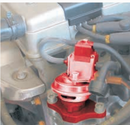
Electric pressure transducer (EDW) on an EGR valve in Opel Astra (highlighted).
