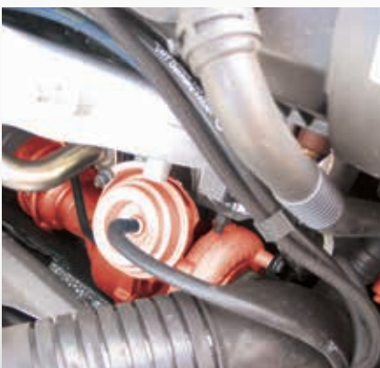
Electropneumatic pressure transducer (EPW) and turbocharger in Audi A4 TDI (highlighted).
