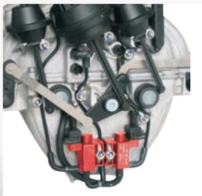
Electric switchover valve (EUV) (highlighted) on the intake manifold of Mercedes-Benz C-Class.
