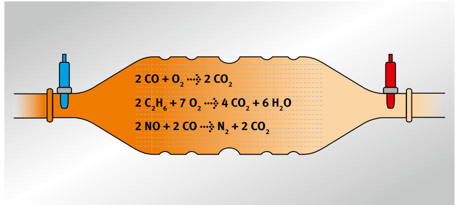
*In regulated 3-way catalytic converters pollutants are rendered harmless by means of three chemical reactions.*
