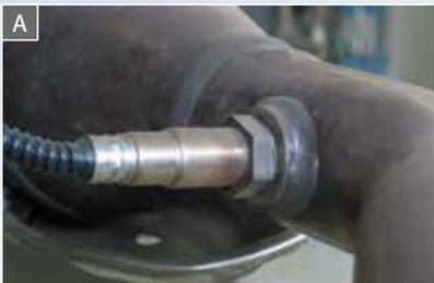
**A** High operating temperatures and aggressive exhaust gas place high demands on lambda sensors
