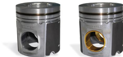
The piston ring set 80 00364 1 1 000 has an oil ring of the third ring groove with drilled profile, as illustrated by figure below:
