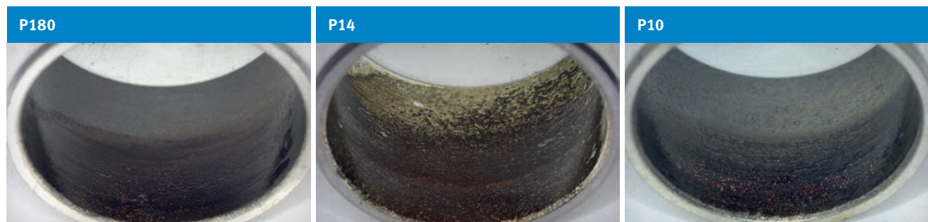
Wear on the sliding layer for P180, P14 and P10 plain bearings after the test rotation in dry running with edge load
