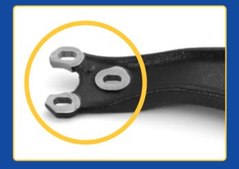
Unlike other designs which have circular holes, the OE lower wishbones of Audi TT 1998-2006 applications have slotted ball joint securing points which allow for camber adjustment.
