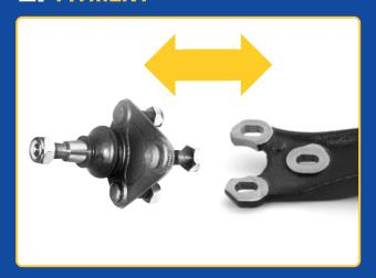
After replacing the ball joint and settling the suspension's weight on the vehicle's wheels, reset both the caster and the toe to ensure proper handling and prevent excessive tyre wear.
